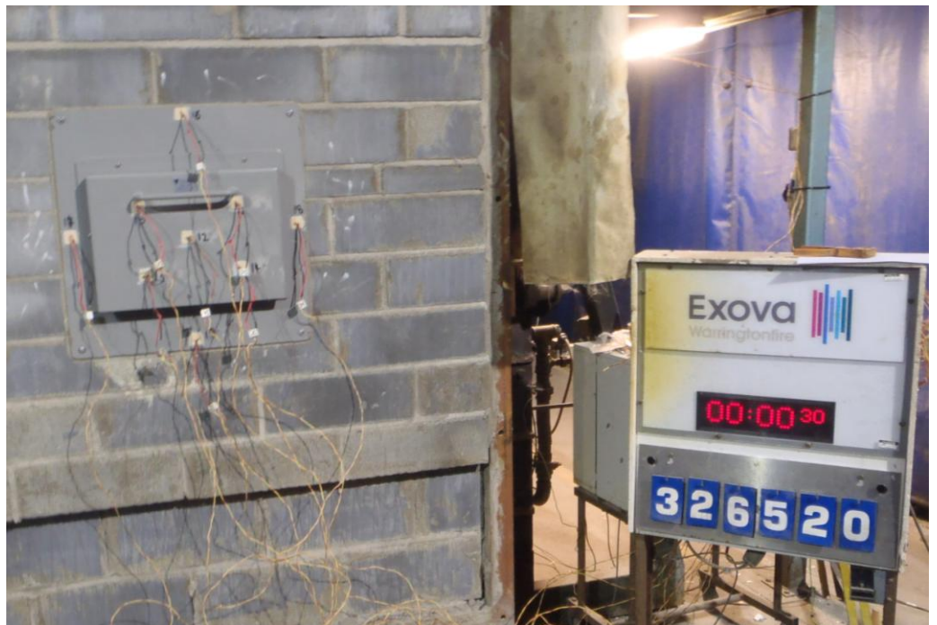
The unexposed face of the specimen prior to testing
