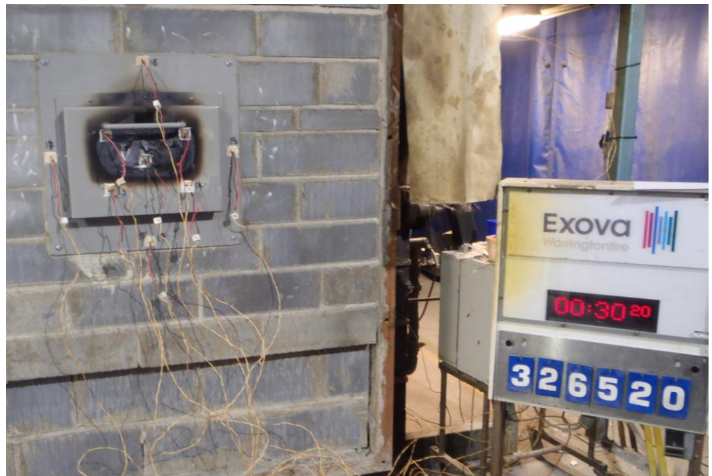
The unexposed face of the specimen after 30 minutes of testing
