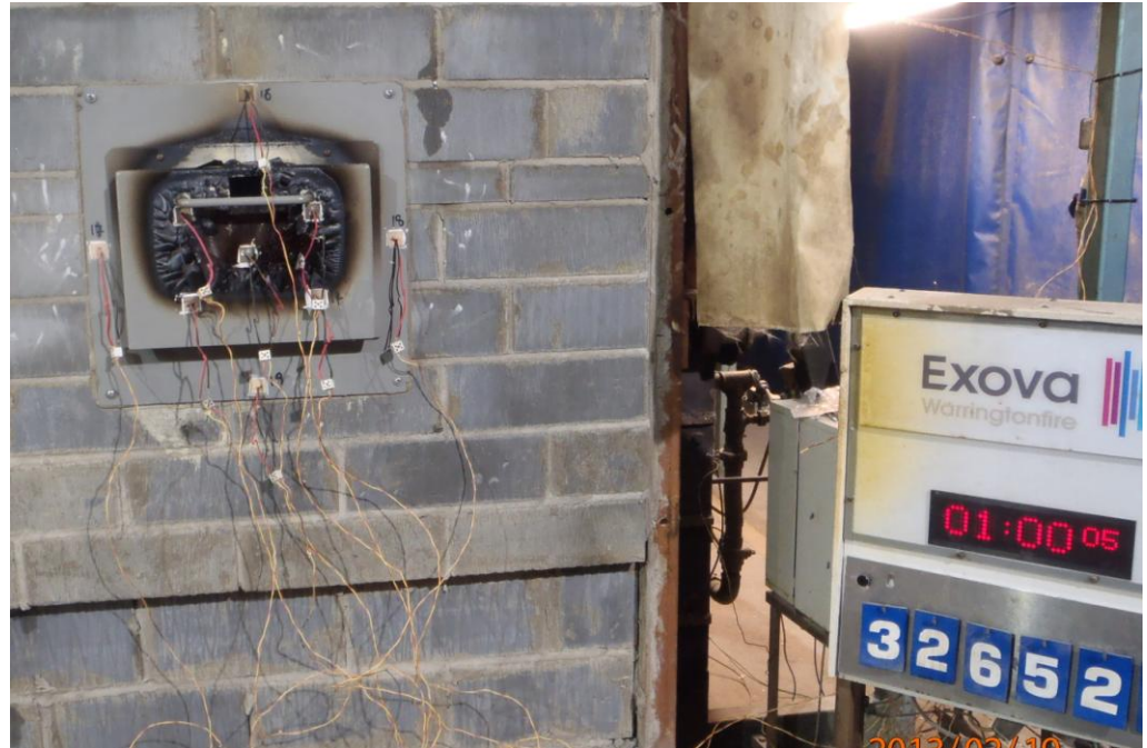
The unexposed face of the specimen after 60 minutes of testing
