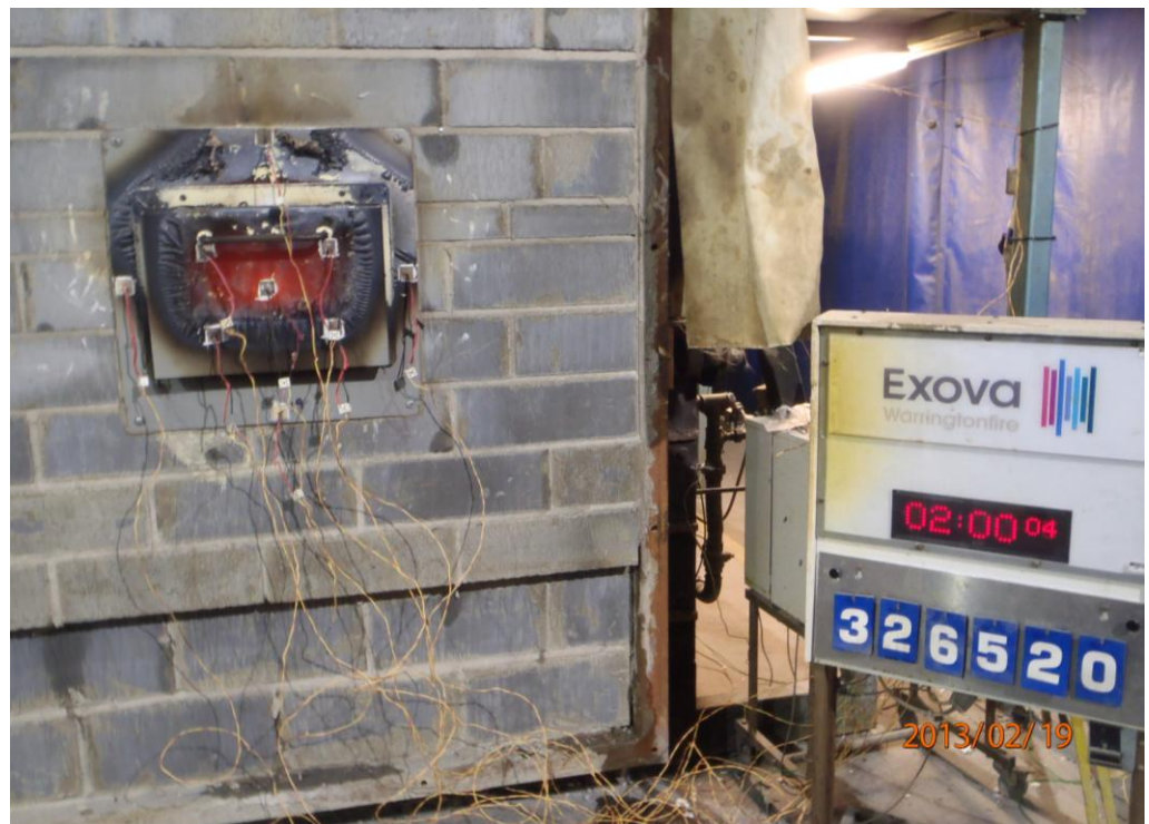
The unexposed face of the specimen after 120 minutes of testing
