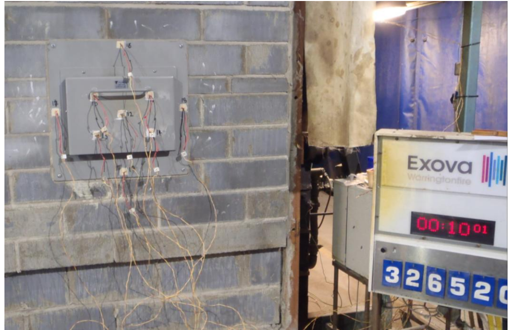
The unexposed face of the specimen after 10 minutes of testing
