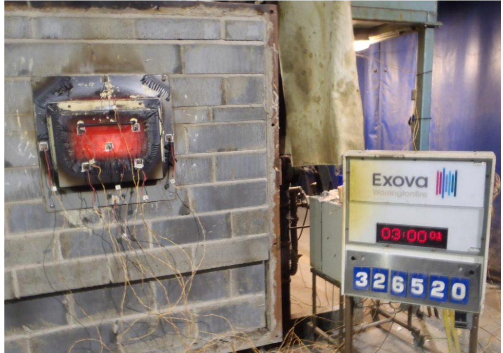
The unexposed face of the specimen after 180 minutes of testing
