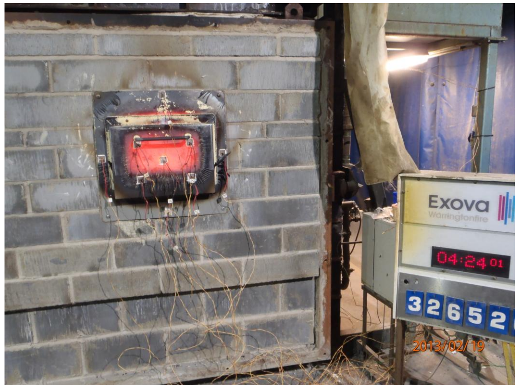
The unexposed face of the specimen after 264 minutes of testing
